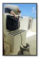
Note: Butane weighs 18% more than propane per liter (or gallon). That means, theoretically, your tank should be full when the weight of the tank is equal to: tare weight + (capacity in lbs of gas x 1.18). A standard 10 lb. aluminum tank from the USA should be full of butane when it weighs 21.8 lbs., not 20.0 lbs. The density of LPG is temperature dependent so these numbers are approximate. Use this information at your own risk.
